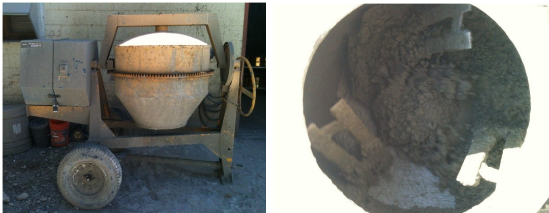
Figure 3.3.2. Concrete mixer and the mixing concrete.
