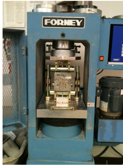
Figure 3.5.3.1. Modulus of rupture testing device with specimen.
