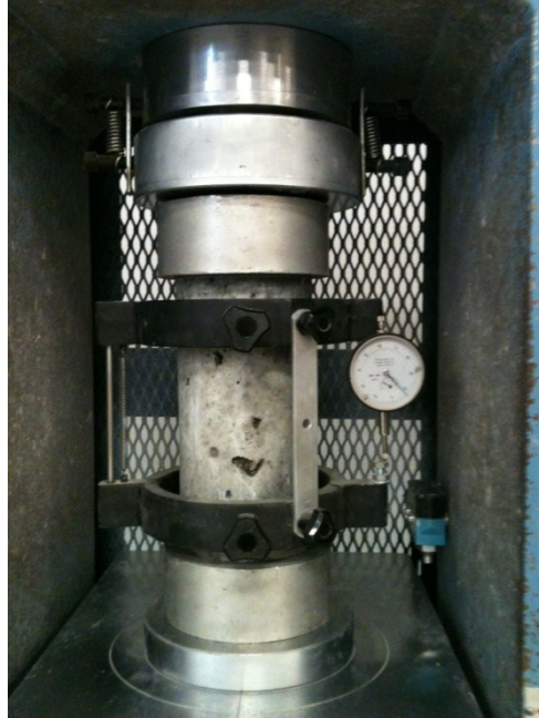
Figure 3.5.4.1. Modulus of elasticity testing device with specimen.
