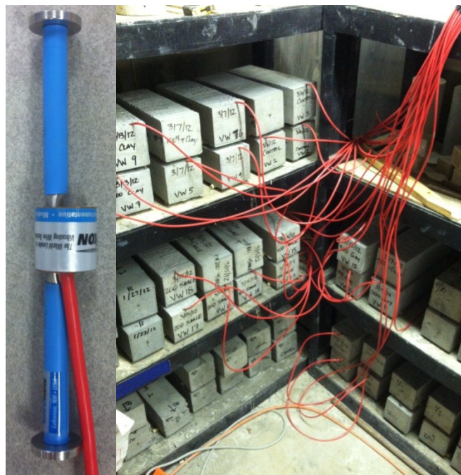
Figure 3.5.2.2.1. Vibrating wire strain gage and specimen storage.
